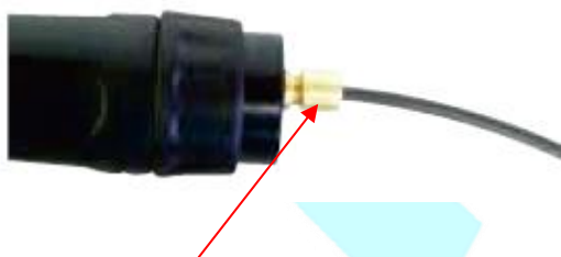
(6) Push the liner firmly into the torch lead and tighten the liner retaining nut.
